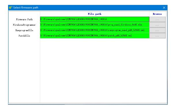
2. Click start button, and then power the module, the tool will automatically detect the module port and start to download
